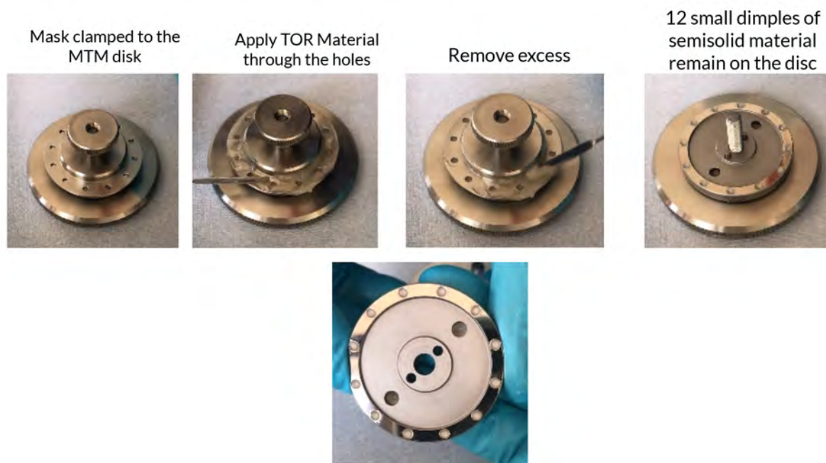
Figure 4: Photographs showing the step-by-step application of semisolid product onto the surface of a MTM disk.
