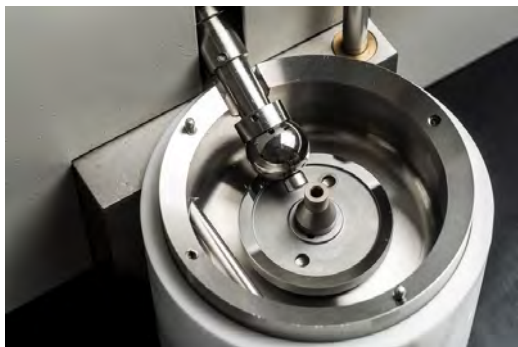
Figure 3: Photograph of the ball and disk attached to the MTM
