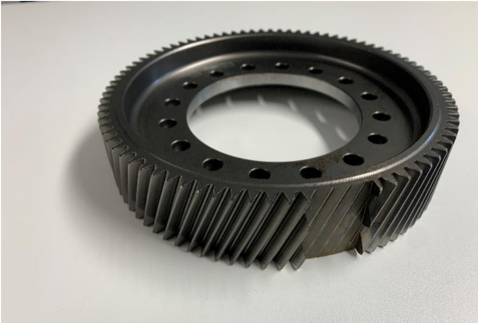
Figure 3 A transmission gear with a selection of teeth removed by a EDM process.
