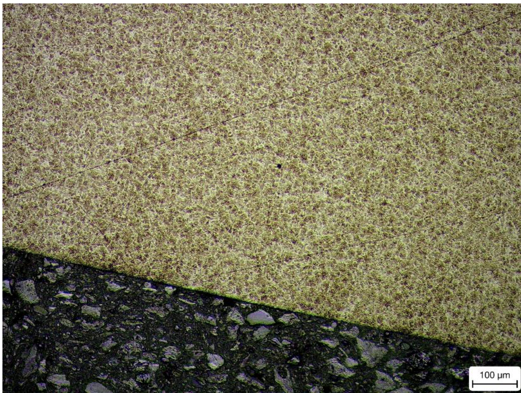
Figure 1 Examples of a subsurface image of the material below the surface of the bearing raceway.
